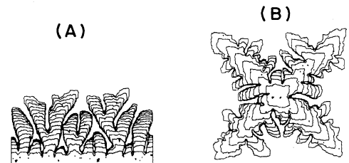
FIG. 5. The effect of the growth geometry on the morphology. The two stroboscopic pictures also show the difference in growth velocity between both morphologies, as the time elapsed between two consecutive snapshots is the same in both plots. ( \omega = 8000 , -\mu_s/T = 2.8 , E_B/T = 2.66 , D = 10^4 , c_\infty = 0.7 , and the system size is 400 \times 400 .) (a) Tip-splitting growth is observed in a channel. (b) Dendritic growth is observed for the same parameter in a channel. The total simulation steps are half of those for (a), as the velocity is much higher.
